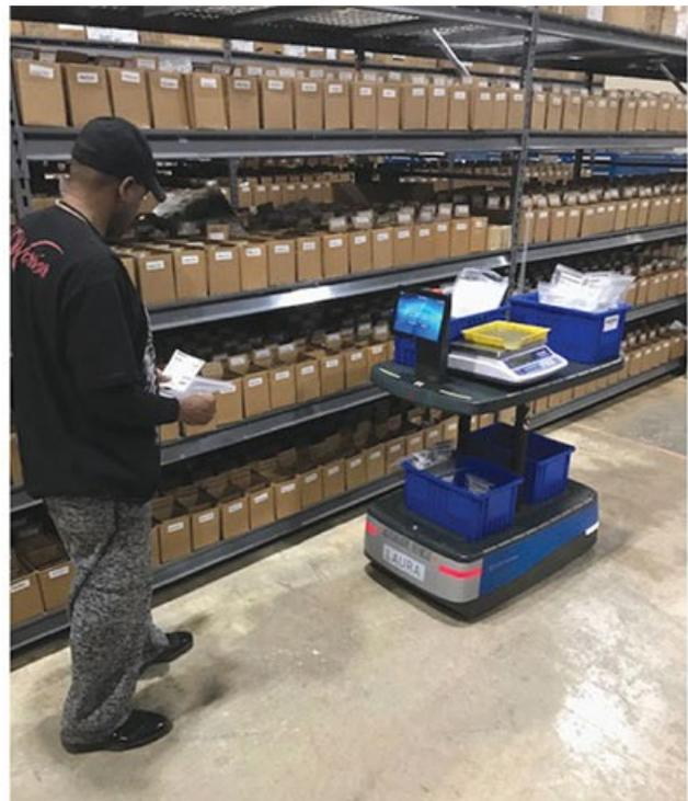
*The Chucks support a directed workflow approach where the bots work alongside human pickers, leading them through the picks along an optimized path, giving them instructions, and transporting completed pick containers to the next point in the fulfillment process.*
